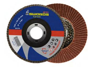
**T-27** - Used for grinding flat surfaces. Most efficient when used at a 0-15 degree angle.
